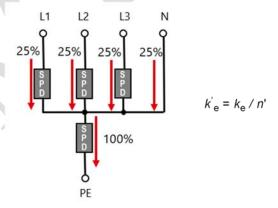
To ensure that the above service conditions are met, a symmetrical current injection as shown in figure 1 is being proposed as an option for the operating duty test of the neutral-to-earth mode. The same approach can be applied for SPDs in 1+1 connection.
